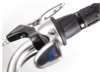
The *Harmony* Advanced Controller offers both fully automatic and manual shifting options in one drivetrain. In “Automatic” mode, *Harmony* automatically and continuously adjusts the drive ratio to maintain the rider's preferred cadence. The Advanced Controller allows the rider to select and fine-tune their cadence set-point by twisting the shifter. *Harmony* will automatically and seamlessly maintain whatever cadence
