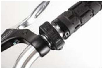
Base Controller intelligently manages the ride by automatically maintaining the pedaling cadence the rider chooses. With its three-button automatic-only shifting, things are kept very simple: press a button and enjoy the ride! The cadence settings (typically slow – medium – fast) can be preset by the e-Bike manufacturer. With the Base Controller, the rider need never think about shifting again.
